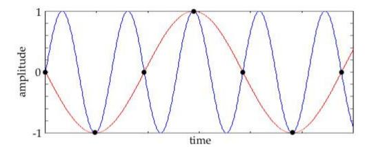
The more wavy line (the higher note) and the less wavy line (the lower note) come together every two vibrations (or cycles). They "fit" like fingers in a glove. Your ear tells you that the two notes are "consonant" or "harmonious". If your piano goes out of tune, the two notes will no longer sound so good as they will not have that 2/1 ratio. The notes would be "dissonant" because they do not fit together any more.
